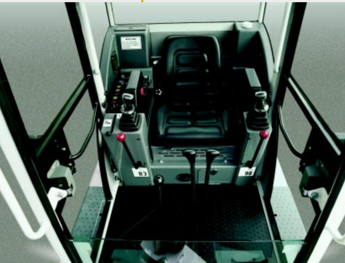
Servo-assisted dual-lever joystick control for all the working functions.
