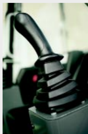
Servo-assisted dual-lever joystick control for all the working functions.
