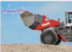
Rugged Z-geometry for enormous breakout forces and high loading speeds.
